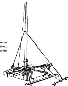
Fig. 43. Construction of the horizontal pit-treadle loom. The transportable parts (cf. fig. 42) have been supplemented by raddle-beam, warp-beam and two small uprights for the breast-beam. The treadles hang down into the pit.
